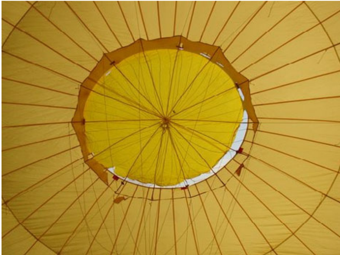
Damaged Parachute on G-BIFC Colt 14A-jpeg Steve Roake
