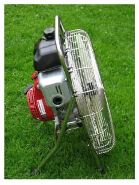
The 3hp engine is the same as the LBL variant, so other than the frame, the biggest difference I could see with the Ultramagic was the 3 tipped plastic blade, as apposed to the LBL/Cameron 6-blade, the efficiency of which is something I have personally never been convinced by. The cost is very similar to Cameron/Lindstrand, being around the £800 mark.
