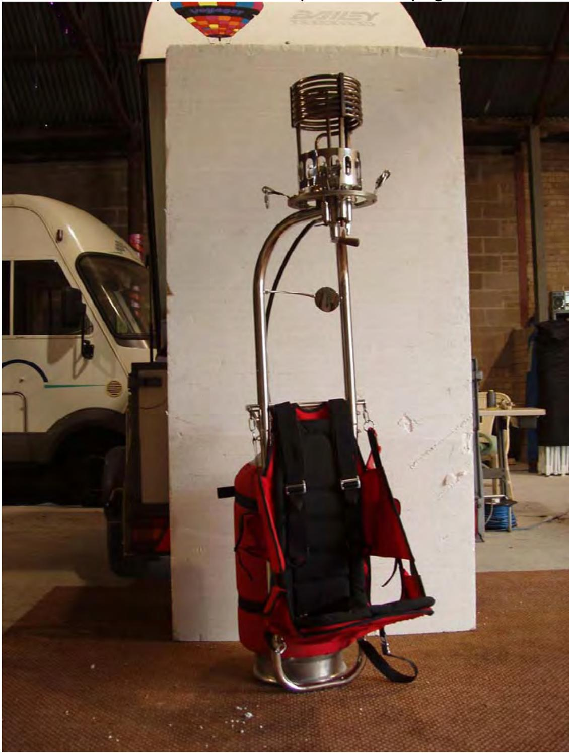
This particular jpeg shows another version with exceedingly long tubes linking the harness to the burner assembly.
