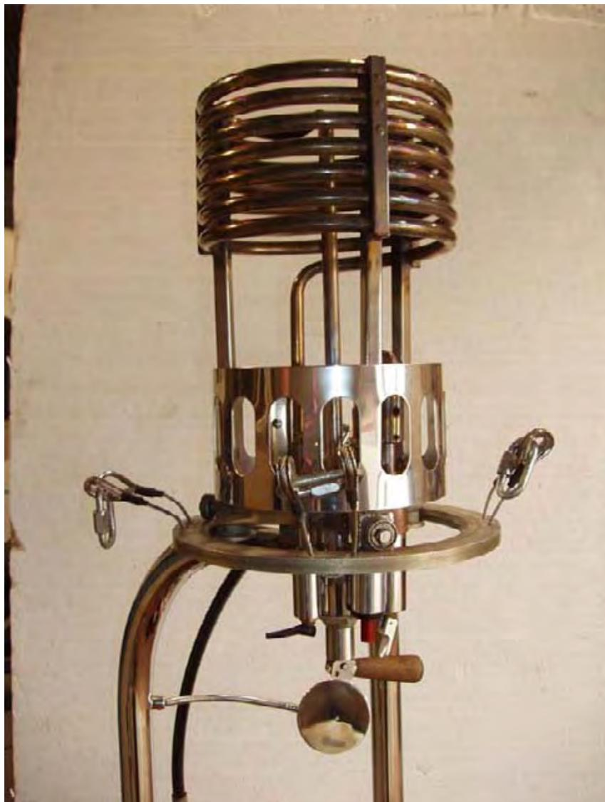
Clearly some thought has gone into the design of the burner on this Mark 2 with the flexible mirror for fuel gauge checks.
