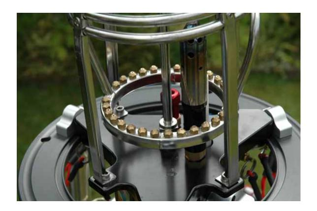
Some three holes to the left hand side are clearly bigger than the others with the next four blanked off. Of note also is the fact that because my Colt 31A has turning vents, the plate that normally spins on bearings is clamped fast in this application.
