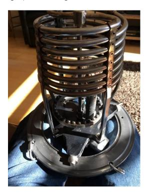
Evidence photograph! note the filed area on the RHS frame where the serial number has been removed, but also the serial clearly evident on the bearing carrier.
