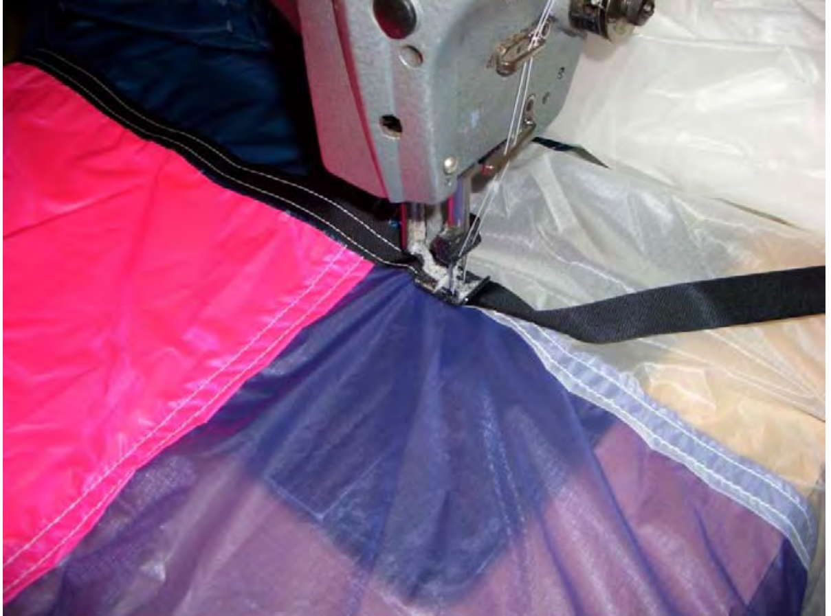
Adding “horizontal” stress tapes to the outside of the balloon.
