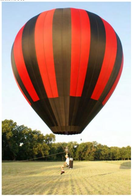
The sewing process went surprisingly fast, and I was able to complete the envelope in about one month. Ripstop Nylon, coated for zero porosity, and weighing 1.8 ounces per square yard, was used for the entire envelope including the 8-foot diameter parachute top. Nomex was used for the lower portion of the
